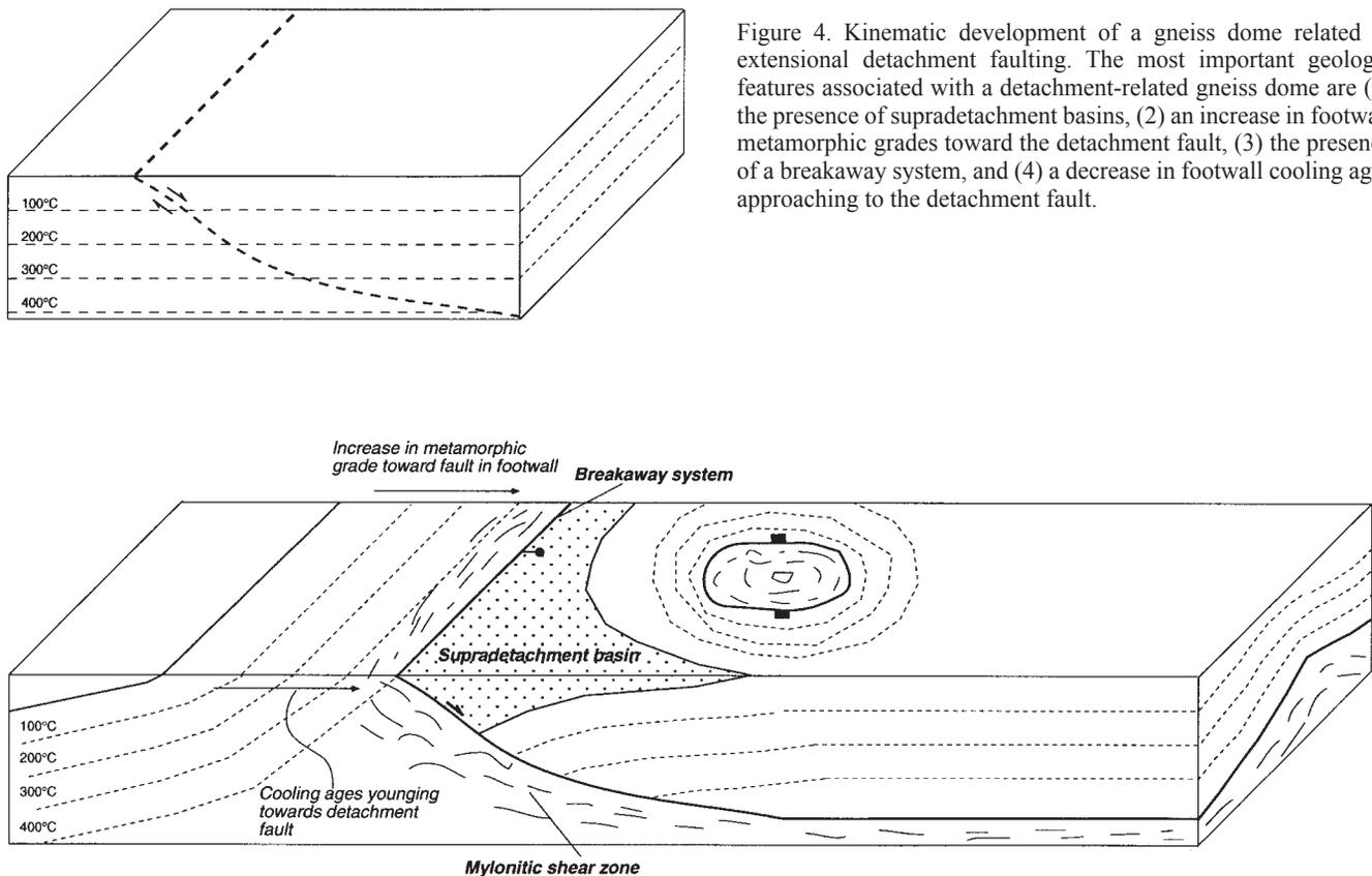
Figure 4. Kinematic development of a gneiss dome related to extensional detachment faulting. The most important geologic features associated with a detachment-related gneiss dome are (1) the presence of supradetachment basins, (2) an increase in footwall metamorphic grades toward the detachment fault, (3) the presence of a breakaway system, and (4) a decrease in footwall cooling ages approaching to the detachment fault.
