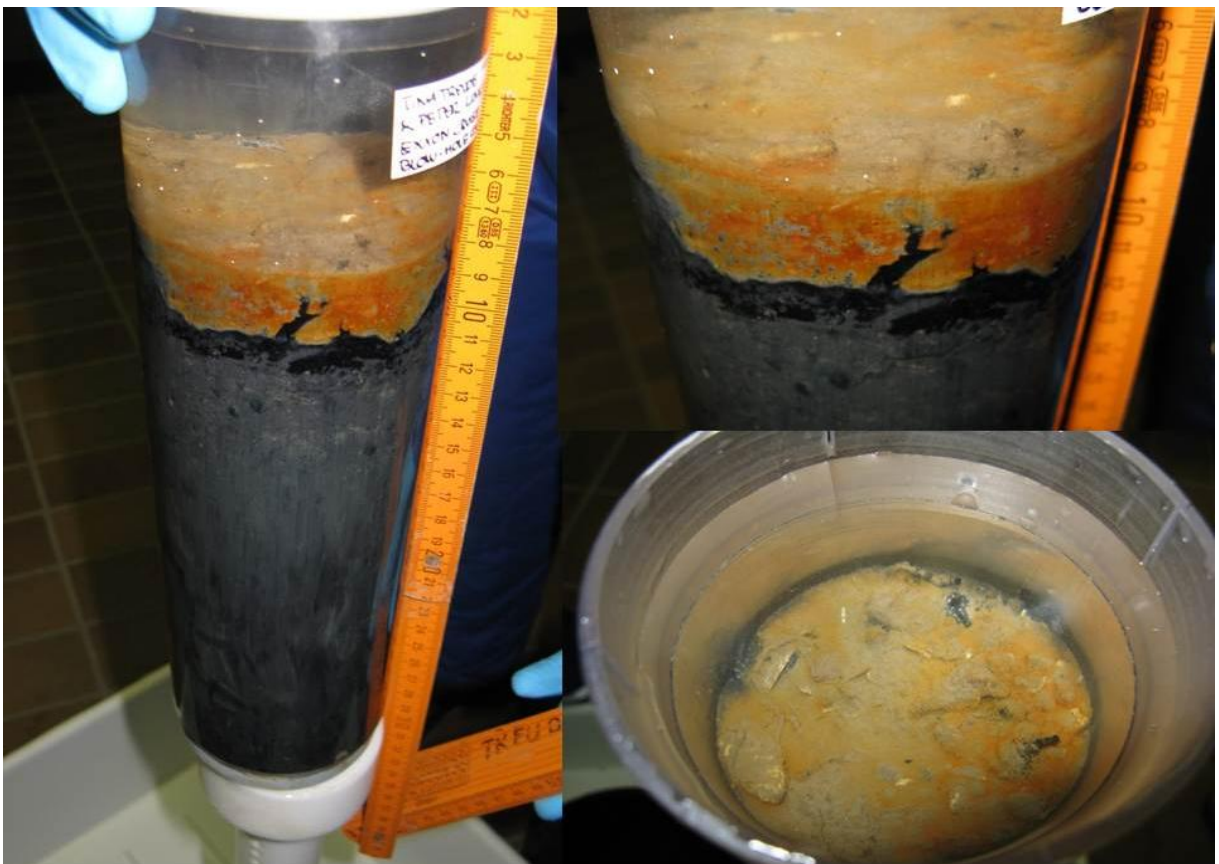
Figure 10: Undisturbed sediment core from the blow-out site in the North Sea. The top of the core was covered with clam shells (bottom right). One can clearly see a distinct oxidized layer where the sediment was in contact with oxygenated seawater (top right). The sediment color below the oxygenated layer was dark grey with some black dots (left).
