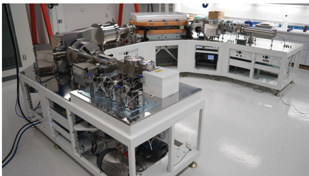
Figure 13.1 Mass spectrometer used to separate the two rare mass-18 isotopologues of CH 4 gas molecules. The instrument – the Panorama – is housed at UCLA and is the first of its kind (Young et al. 2016).
