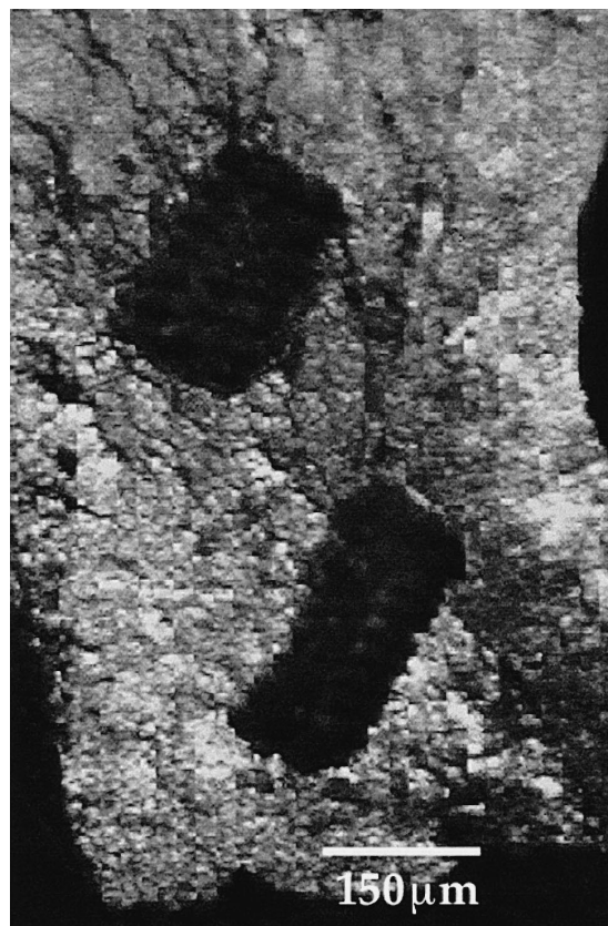
Fig. 3. Photograph showing UV-irm-GCMS laser ablation pits in sample ICT1.
