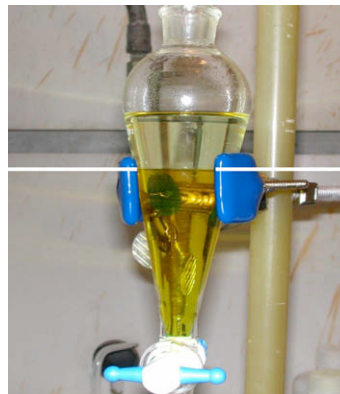
Fig. 2. Separation of ether and aqueous phases in a ferric chloride solution. The ether phase is on the top.
