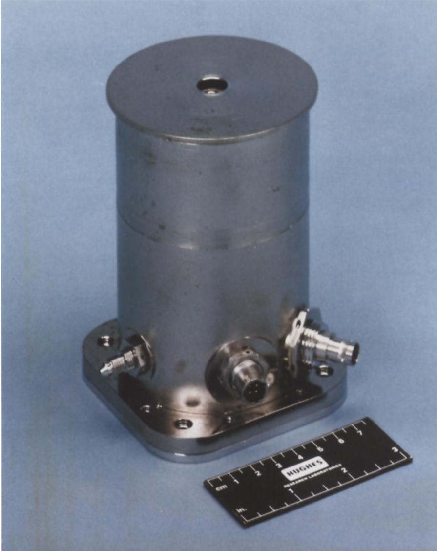
Plate 2. Photograph of the PSI source assembly. Plasma is emitted from the aperture at the end of the cylindrical package.
