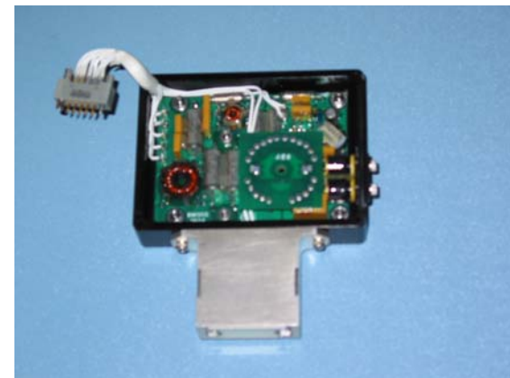
Low Voltage Power Supply
