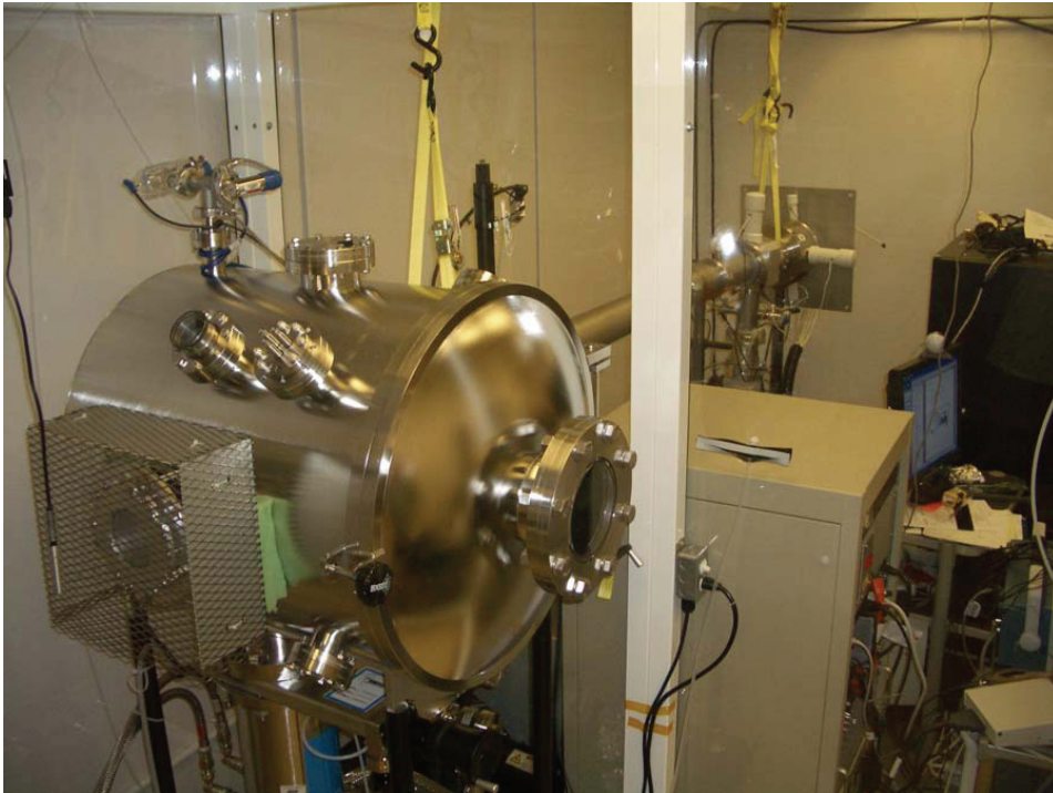
Figure A.73: One of the University of California, Berkeley vacuum calibration chambers. The near side of the 30 inch chamber has an UV photocathode gun [Lessard et al. , 1998] that provides a 10 cm electron beam at energies up to 30 keV. On the opposite side of the chamber is a Peabody Scientific mass selectable ion source, with drift tube to reduce background, and an energy range of 2 to 50 keV. Having both guns on the same chamber facilitates testing of instruments that contain both ion and electron detectors. The vacuum chamber and electron gun reside inside the clean room while the ion gun extends into the outer room for easy access.
