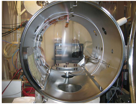
Figure A.81: Internal view of vacuum chamber, showing instrument turn table.
