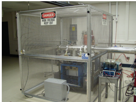
Figure A.78: Ion accelerator system for the University of Michigan's MASS SPEC Laboratory. The system provides an ion beam with an energy of up to 30 keV.
