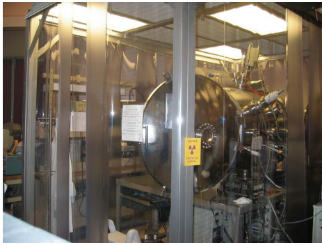
Figure A.80: University of New Hampshire Space Plasma Experiment Testing Facility: Vacuum chamber in class 10K clean tent.
