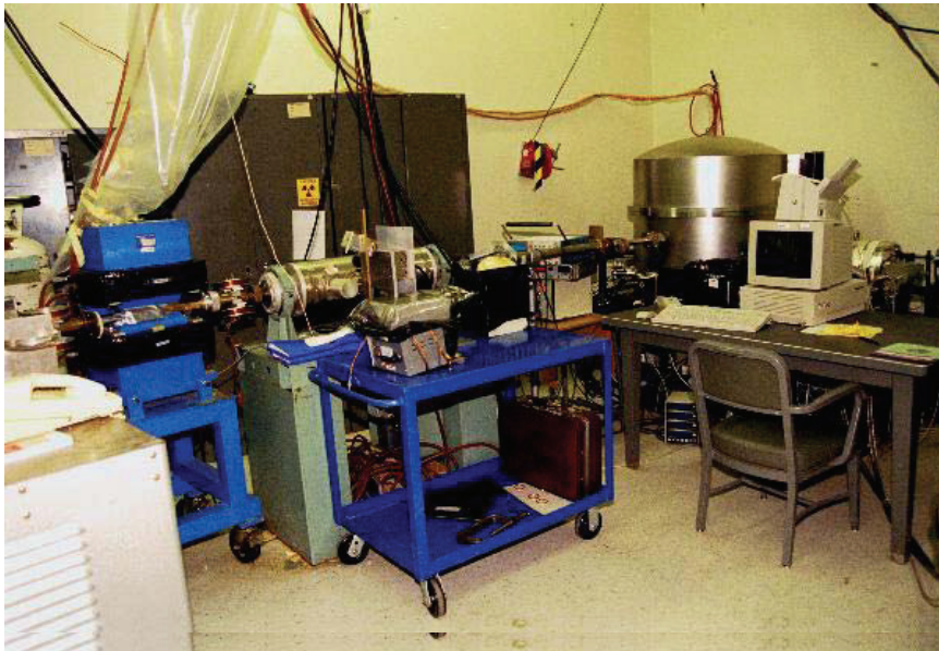
Figure A.21: Radiation Effects Facility (GSFC REF) steering magnet, electrostatic focus and 76.2 cm D \times 96.5 cm H test chamber for the instrument Van de Graaff.
