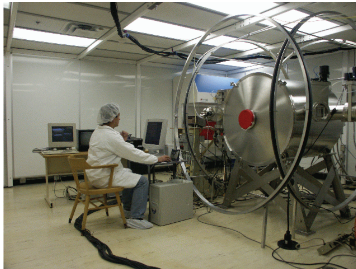
Figure 3.5: Electron beam calibration facility of the University of Calgary, Canada. View of vacuum system from inside the cleanroom with the Helmholtz coil system. For details see Appendix A.4.
