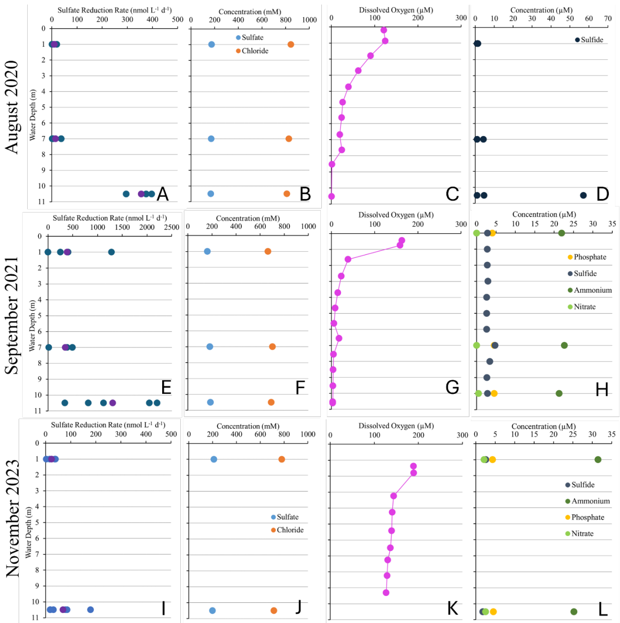
Figure 4-2. Biogeochemistry of the Salton Sea water column during three sampling campaigns (top: August 2020, middle: September 2021, bottom: November 2023). (A, E, I): Sulfate reduction rates. Blue dots represent individual measurements while purple dots represent the average. Note the change in scale for E compared to A & I. (B, F, J): Sulfate and chloride concentrations. (C, G, K): Dissolved oxygen concentrations. (D, H, L): Phosphate, sulfide, ammonium, and nitrate concentrations. Note the change in scale for D compared to H & L.
